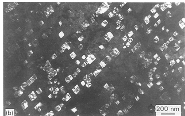
Figure 5 Scanning electron micrograph showing a grid of secondary carbides after 0.25 h at 1273 K.
